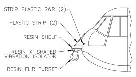
frame. This shelf is supported by two angle struts which span the small door in the nose. These can be represented by 0.020" x 0.020" square strip. Below the shelf, glue the isolator (flat side on top), then the turret. The mounting arms really are slanted slightly forward, so don't try to straighten things up! The IR sensor ball is given in its normal stowed position with the lens facing the aircraft. The shelf and supports are airframe colour, while the vibration isolator and
