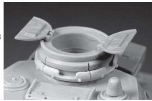
This photo shows the assembled open cupola with gap forward (here seen on a PzKpfw IV)
