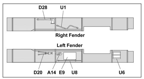
the fender of the kit upper hull, and place it where you desire. Replace cover plate F3 with resin parts 6 and 7. The one with the small bar goes in front. Replace rear cover plate E17 with resin part 8. The cover plates E12 are not required, neither are the spare roadwheel mounts E7. One towhook (parts A14) and box E9 will be relocated according to sketch.
